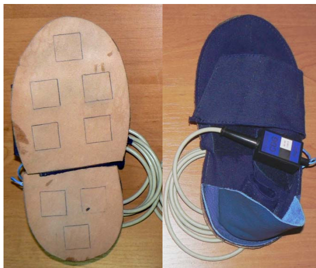
Figure 1 The shoes (Computer Dyno Graphy (CDG) ® system Infotronic, Netherlands). Shown is the bottom of the leather sole containing the 8 sensors, and the elastic upper.
